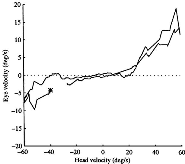
Figure 4. The  $xy$  plot of a soft dead-zone nonlinearity at 0.03 Hz. This type of nonlinearity was often observed with habituation at 0.01 Hz but was more pronounced at slightly higher frequencies (0.03 and 0.05 Hz). The asterisk indicates the start of the cycle. The soft dead-zone  $xy$  profile is characteristic of the magnitude-dependent VOR response.
